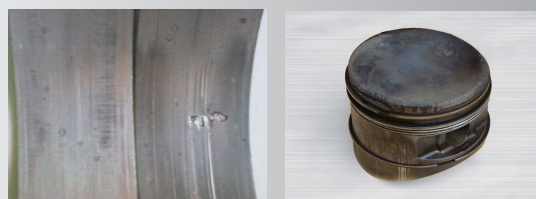
Hammered bearings (left) and damaged piston (right) due to prolonged engine pinging & detonation.
